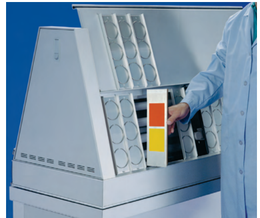
Standard sample holder is installed by resting it in a slot on the QUV frame. To seal in vapor, it is essential to operate with all holders in place and with blank panels in all unused spaces.
