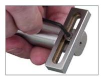
a. The actual wet film thickness will depend on the behaviour of the wet coating.
